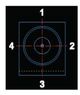
Orientations are called out by three position number (e.g. 110) looking at the actuator from the front with the mounting block as shown:
